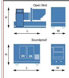
Open Type (Standard Configuration) Overall Size: 4600\*2190\*2290 mm(L\*W\*H) Weight:7150Kgs
