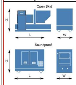
Open Type (Standard Configuration) Overall Size: 5800\*3000\*3150mm(L\*W\*H)
